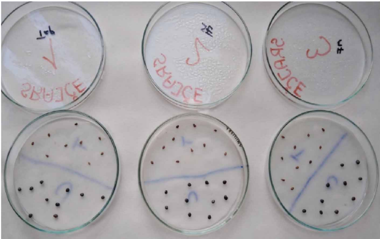
Figure 1 | Seeding of tomato and cabbage seeds with tap water, secondary effluent, and membrane effluent. Lower-row Petri dishes contain the seeds, and the upper-row Petri dishes were used as lids to ensure a high humidity environment. Inside the lower-row Petri dishes are paper media on top of which lies the seeds. Each lower-row Petri dish is divided into two sections (T and C), C represents the section for the cabbage seeds and T is the section for the tomato seeds. The relatively bigger seeds are the cabbage seeds, and the relatively smaller seeds are the tomato seeds. All papers placed in the lower dishes were soaked with the respective irrigation water stream, tap water, secondary effluent, and membrane effluent before the seeds were placed on them. The labels 1 (Tap), 2 (SE), and 3 (ME) on the lids represent the Petri dish for Tap/SE/ME treatments, respectively.
