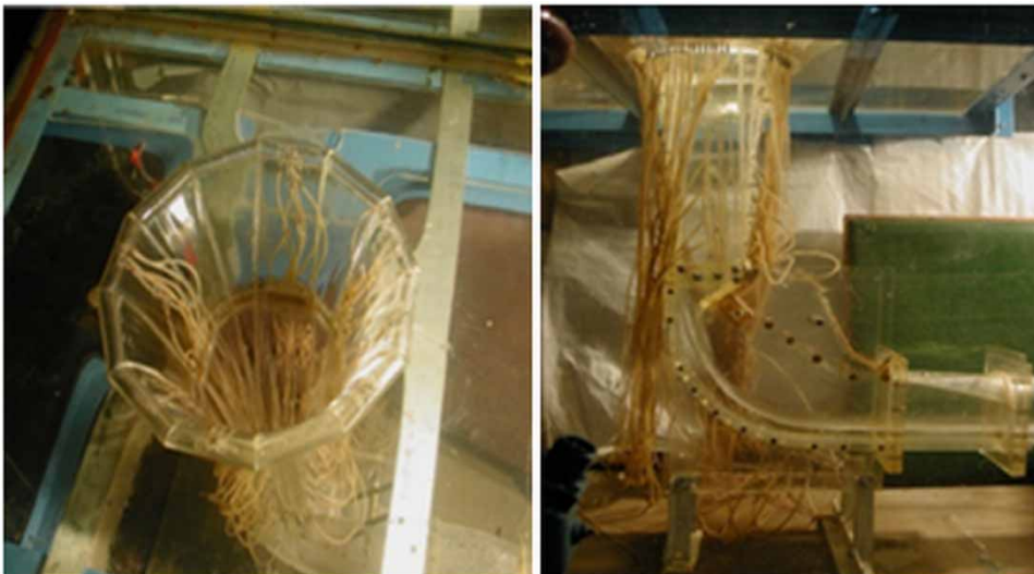
Figure 6 | Photos of the experimental device with the distribution of the piezometers on the model.
