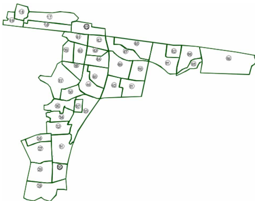
Figure 4 | Ramnagar ESR operational hydraulic zone showing 38 sub-zones.
