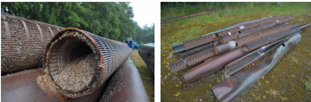
Figure 8 | Pictures of recovered copper screen (150 mm diameter, with stainless steel wire-wound screen insert) and casing from Well 29, Wildeshausen (photographs: Sander).
