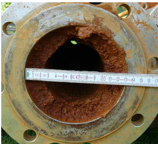
Figure 2 | Typical examples of iron oxide deposits in a riser pipe (125 mm diameter) and on a submersible pump of the Großenkneten well field after roughly six months of operation.
