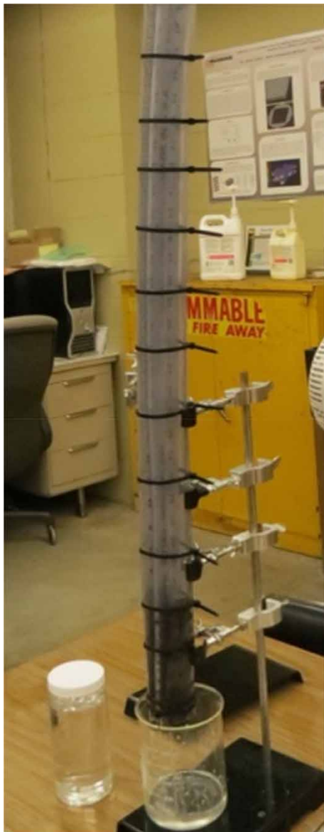
Figure 4 | The final layout of the proposed gravity-based low-cost arsenic filtration system attached to a vertical metal ruler to allow for maximum gravitational force to act upon the passing liquid. The water, poured at the top for creating a certain column above the sponge, was collected at the bottom after its seepage.
