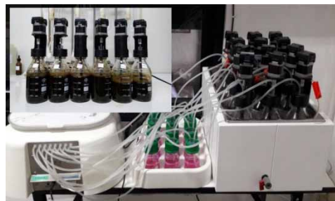
Figure 1 | Automatic anaerobic digestion methane potential test system.
