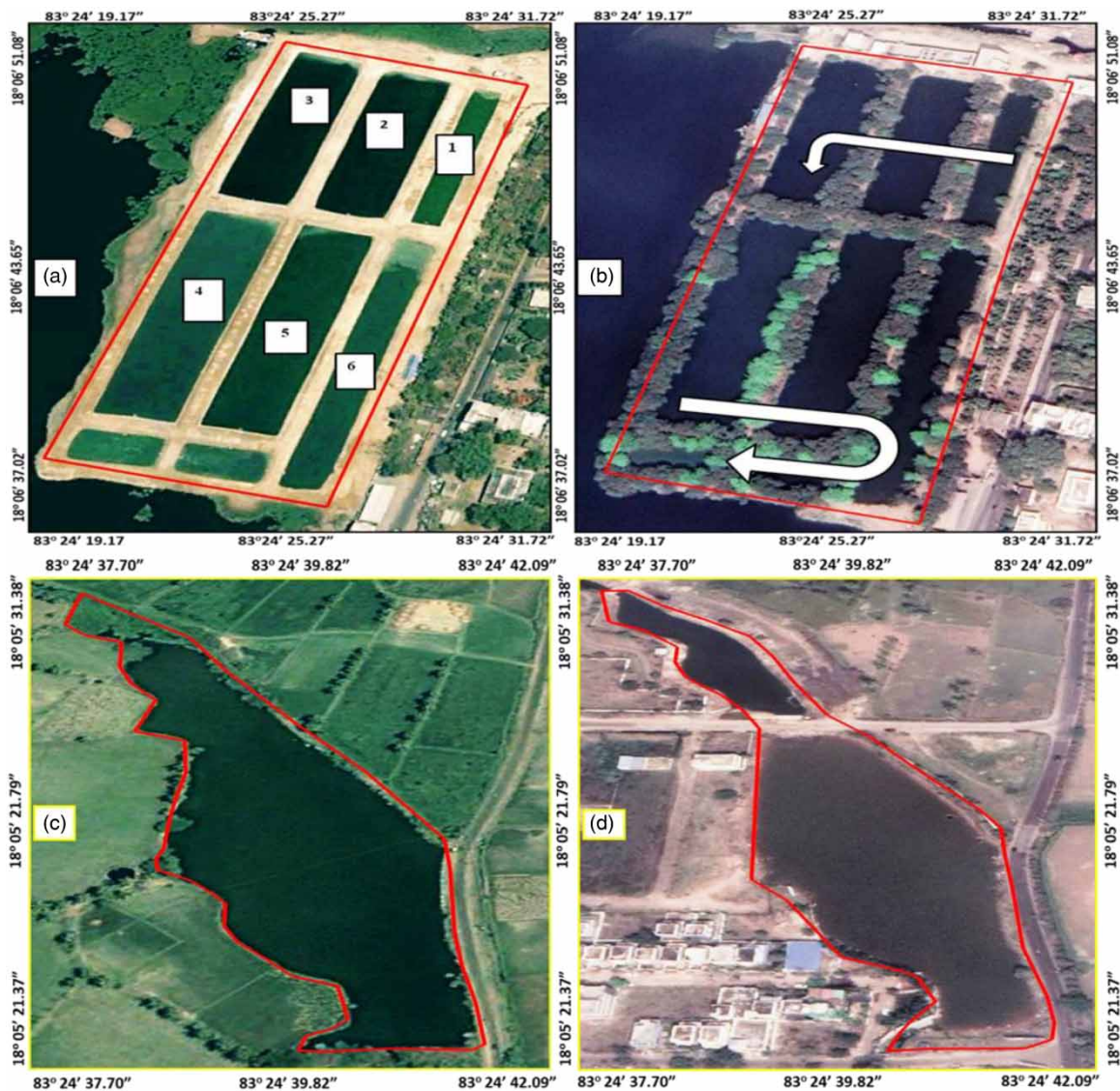
Figure 2 | Google Earth clips and field photos showing the status of the treatment systems NTS 1-4 during the period 2004–05 (left column) and 2020–21 (right column). (a, b) – NTS-1 Waste Stabilization Ponds [1, 4 – Anaerobic Ponds, 2, 5 – Facultative Ponds and 3, 6 – Aerobic Ponds], (c, d) – NTS-2 Hyacinth and Duckweed Ponds. (e, f) – NTS-3 Hyacinth and Duckweed Ponds, (g, h) – NTS-4 Waste Stabilization Ponds [1 – Anaerobic Pond, 2 – Facultative Pond and 3 – Aerobic Pond]. (Continued.)
