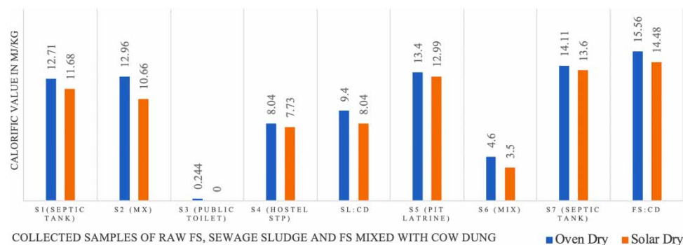
Figure 3 | Variation in calorific values corresponding to different drying and mixing conditions in MJ/kg.
