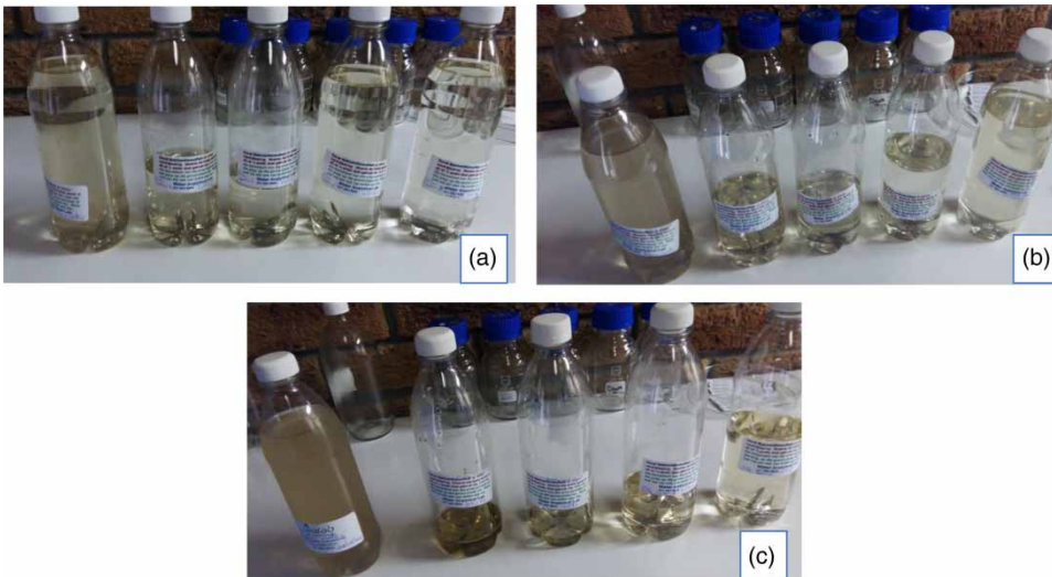
Figure 3 | Raw water and corresponding treated effluents: (a) fresh wood, (b) wet preserved wood and (c) dry preserved wood.
