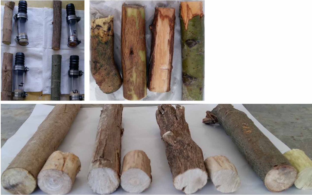
Figure 2 | Fresh wood (top left), wet preserved wood (top right) and dry preserved wood (bottom); Combretum erythrophyllum , Tarchonanthus camphoratus , Leonotis leonurus and Salix mucronata left to right, respectively.
