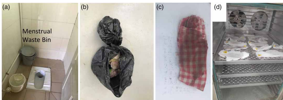
Figure 1 | (a) Photograph of a bathroom stall with individual waste bins. (b) Waste bin bag liner as received. (c) Disposed of homemade cloth pad. (d) Individually labeled commercial pads in a dry oven for moisture measurement.
