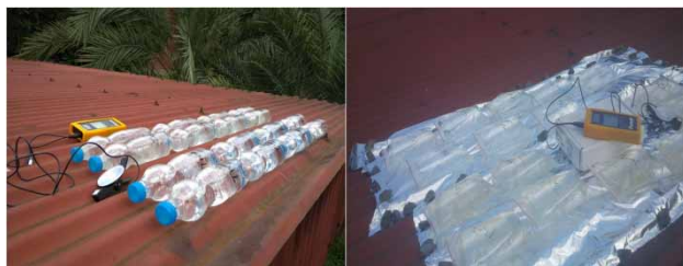
Figure 1 | Reactors used in the SODIS experiments: transmissive (left), PET bottle and reflective (right), plastic bag backing with food graded foil paper.
