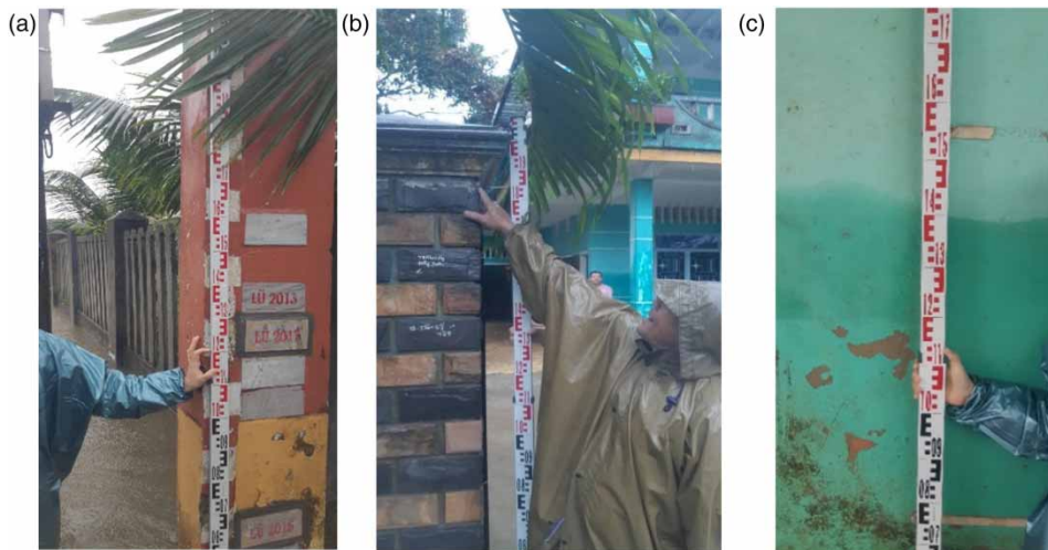
Figure 4 | Measuring the flood location and depth during the field survey in 2020: (a) measuring location and depth at the flood pillar point; (b) asking local people about the severity and contributing factors to local flood; and (c) measuring flood location and depth inside the household.
