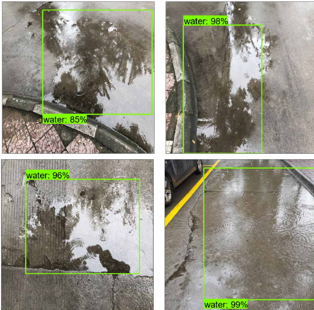
Figure 12 | Actual road inundation detection results. Please refer to the online version of this paper to see this figure in color: https://doi.org/10.2166/hydro.2021.156 .
