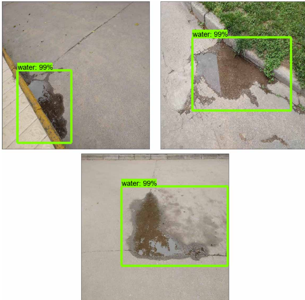
Figure 11 | Experimental road inundation detection results. Please refer to the online version of this paper to see this figure in color: https://doi.org/10.2166/hydro.2021.156 .
