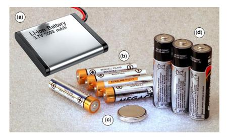
Figure 4.3 Different types of batteries: (a) lithium-ion batteries, (b) alkaline batteries, (c) button cell and (d) Ni-zinc batteries.
