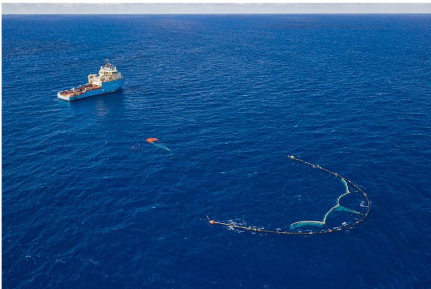
Figure 11.37 The Ocean Cleanup System 001 for marine plastic debris collection (The Ocean Cleanup, 2018).
