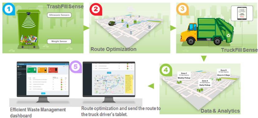
Figure 11.22 An example of commercialized smart Bin and smart waste collection system (Source: modified from Faststream Technologies, 2021).
