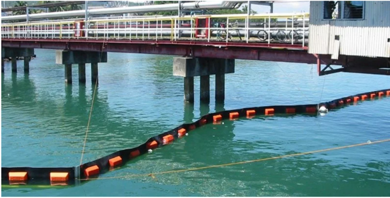
Figure 11.35 Marine litter containment floating boom developed by the CLAIM Project. (Source: Credit: CLAIM)
