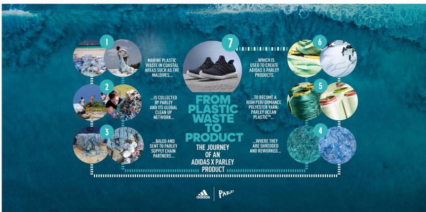
Figure 6.41 Process of making a Parley for the Ocean Adidas product (Source: https://www.adidas.co.th/en/blog/639412-how-we-turn-plastic-bottles-into-shoes-our-partnership-with-parley-for-the-oceans ).
