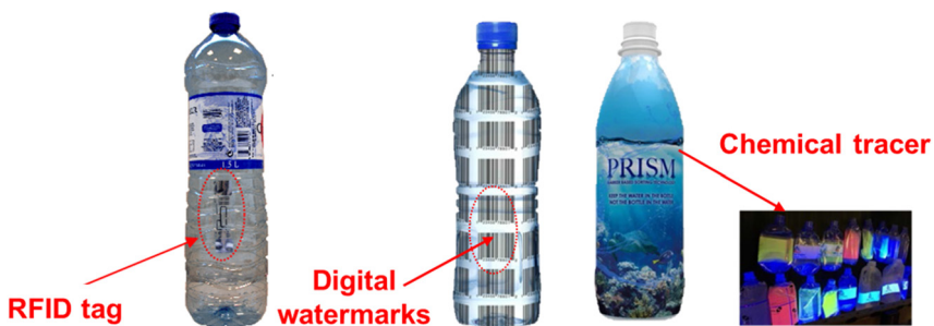
Figure 11.17 Digital tagging technologies applied for plastic waste identification (Sources: Amritkar, 2017; New Plastics Economy, 2017).
