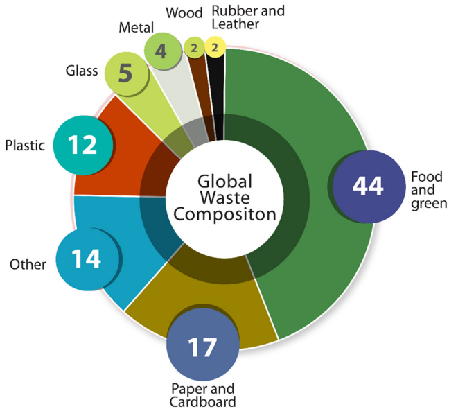
Figure 8.3 Global waste composition and share of plastics in MSW (in %) (Source: modified from Kaza et al. , 2018).
