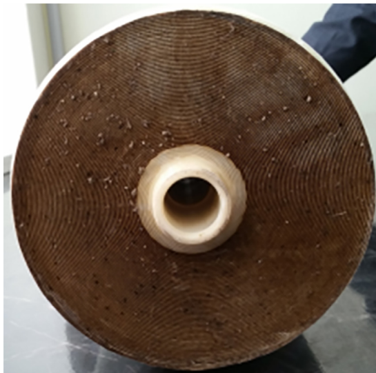
Figure 3.4 Bio-fouled spiral-wound RO membrane.
