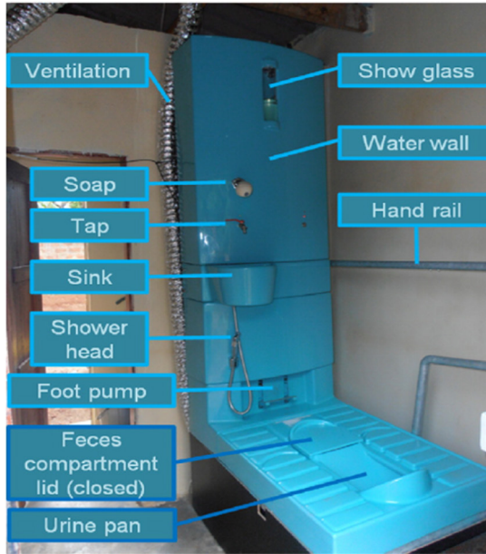
Figure 3.11 The working model of the Blue Diversion Toilet as used in the Kampala field test. The water wall contains the water tanks and bio-reactor. The metallic tube (labelled ventilation) is part of the active ventilation of the faeces compartment to prevent odour. (From Tobias et al. (2017) under CCA 4.0 license, © 2016 by the authors.)
