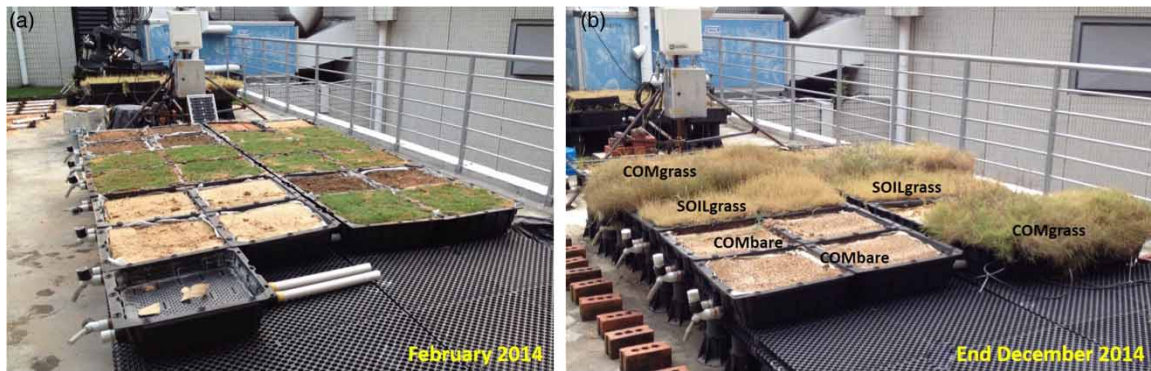
Figure 5 | The green roof design configuration units in (a) February 2014 and at the (b) end of the monitoring period showing that grass is well established on the configuration units.
