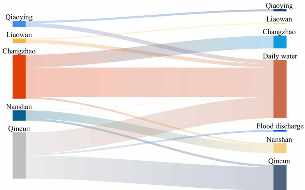
Figure 6 | 2022 Sankey diagram showing the network's joint regulation of regional reservoir group water resources.
